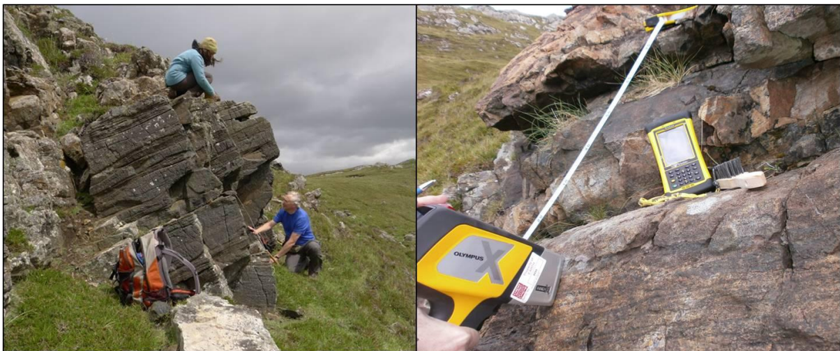
Layering in ultramafic body at Camas nam Buth, Scourie (Drs Hughes and Faithfull for scale). Hand held XRF analysis of ultramafic layers and garnet granulite country rocks.
